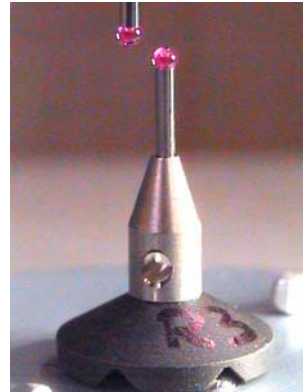
Figure 3 : picture of two of the sapphire spheres being measured against each other
