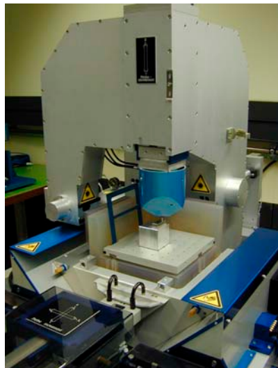
Figure 1 : The ultra-precise coordinate measuring machine ( \mu CMM) at METAS
